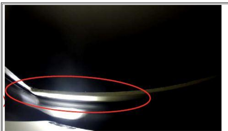
Figure 2: Hood misaligned with respect to Boot seal
