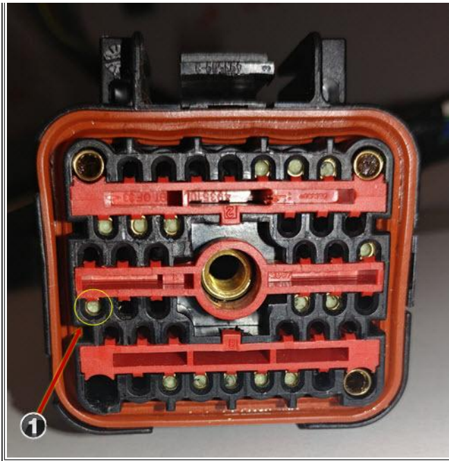
1. Terminal fully installed, body lock had been re-installed
