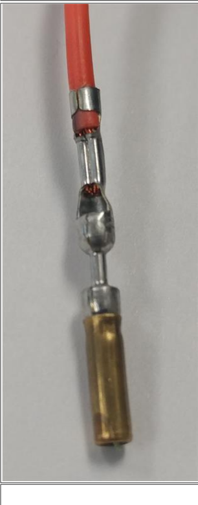
Figure 3: Terminal Properly Crimped
