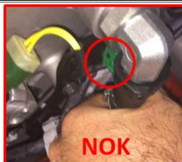
Figure #2: Improper positioning of the coolant line locking retainer. Retainer must NOT be facing the engine.
