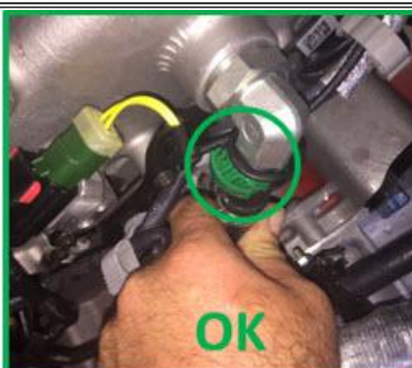
Figure #3: Proper orientation of the locking retainer facing away from the engine.
