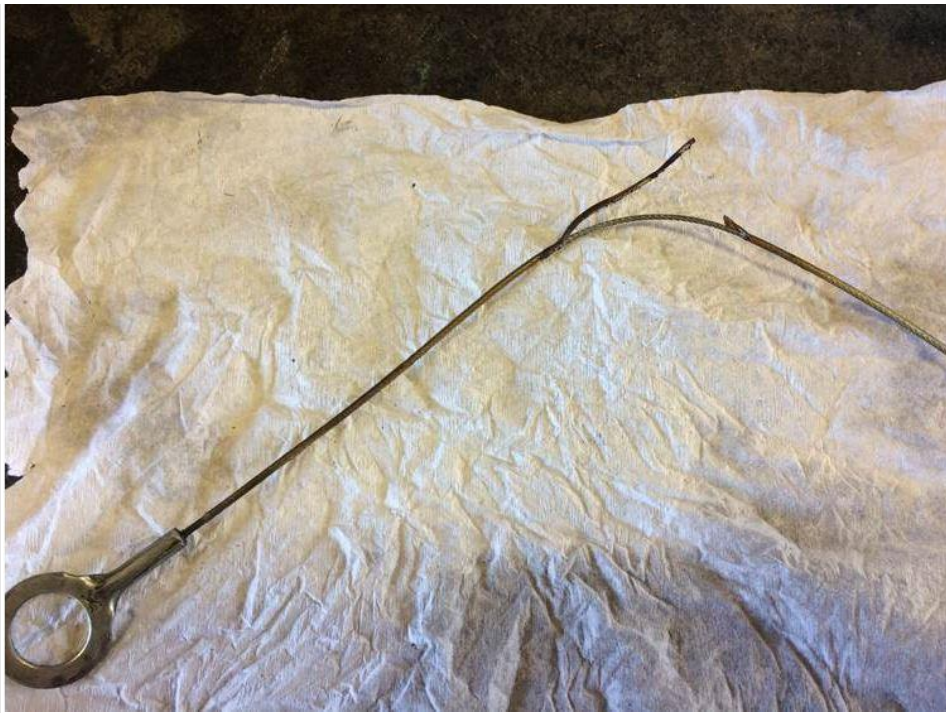
Figure #3: Damaged Cable
