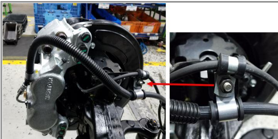
Figure #3: Correct routing and clipping if the brake hose was rubbing, but is NOT damaged. NOTE that the brake hose is clipped under the ABS harness.
