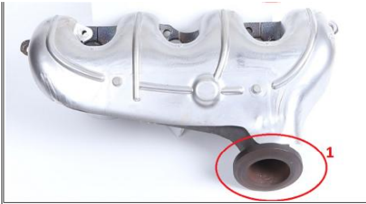
Figure 1. Potential Leak Point
