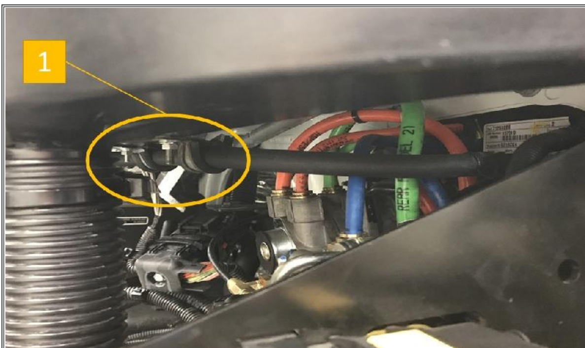
Figure 2. Correct Master Cylinder Supply Hose Routing
