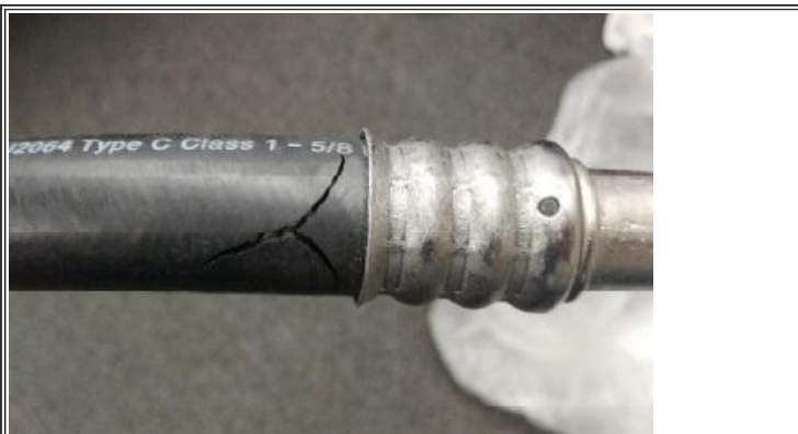
Figure #:1 Sample cracked A/C hose evaporator to compressor
