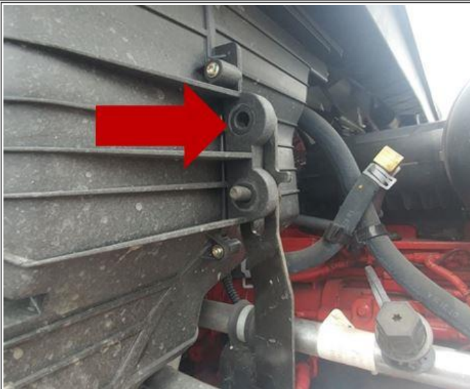
Figure #3: A/C hose support bracket bolts
