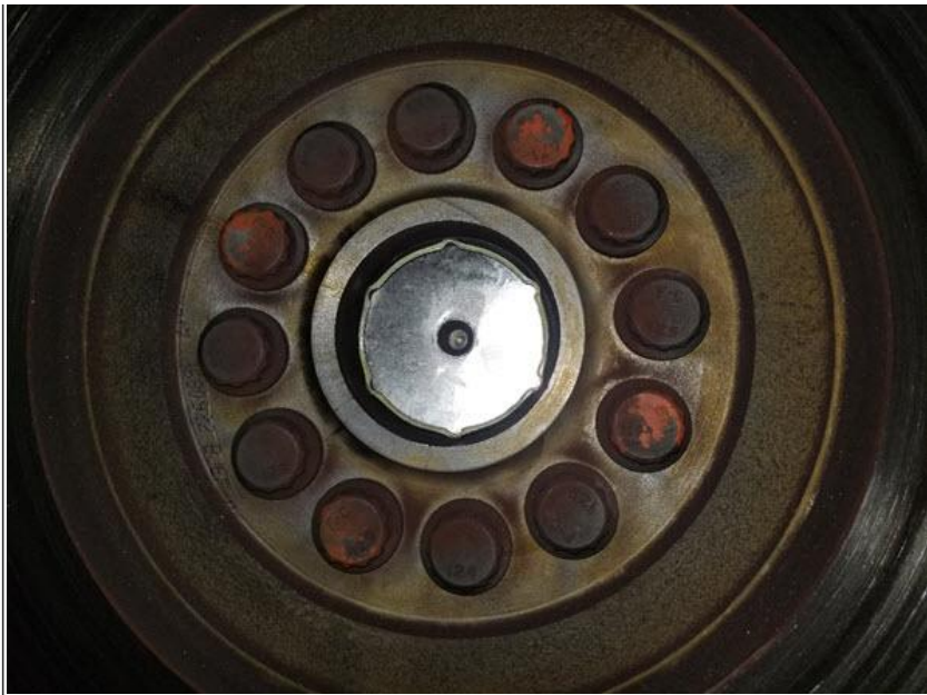
Figure #1: Flywheel Missing Pilot Bearing
