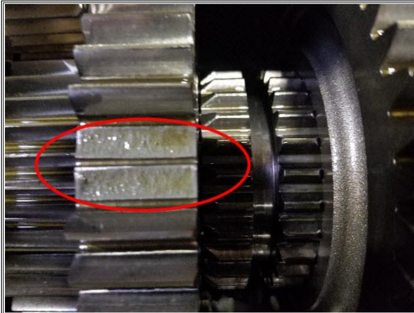
Figure #3: Damaged Transmission Gear
