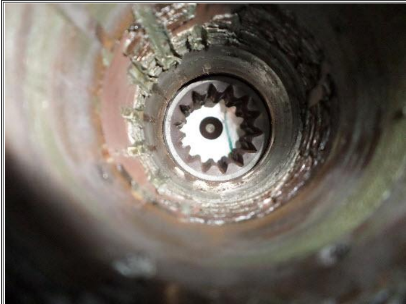
Figure #2: Missing Pilot Bearing w/ Clutch Installed
