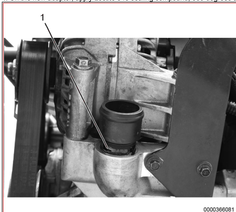
Figure 2 Oil Filler Adapter Sealant Application
