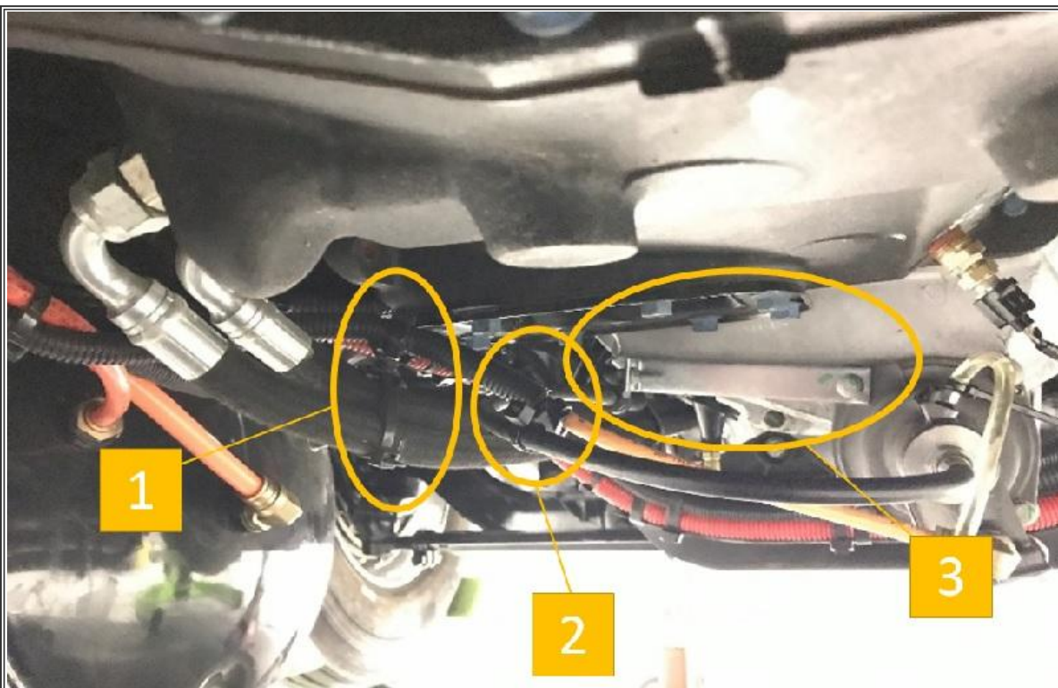
Figure 5. Correct air assist servo Cylinder Supply Hose Routing
