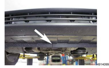
3. Locate the center seam on the front bumper fascia air deflector.
