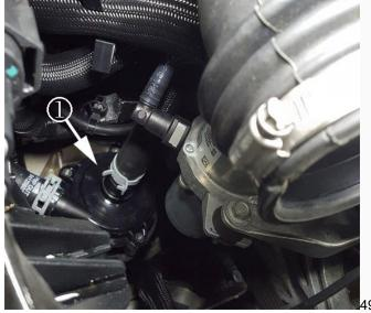
Use the Charge Air Cooler Coolant Pump (1) as a reference point.
