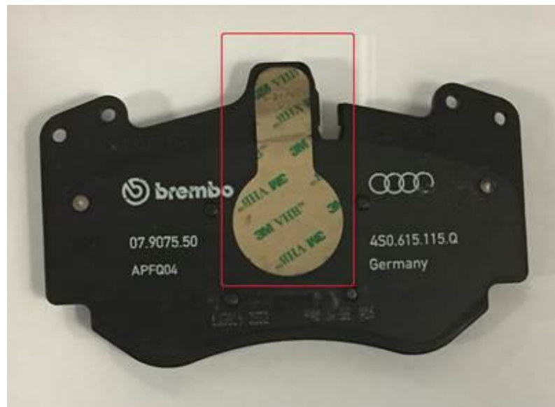
Figure 2. Pull of adhesive foil.
