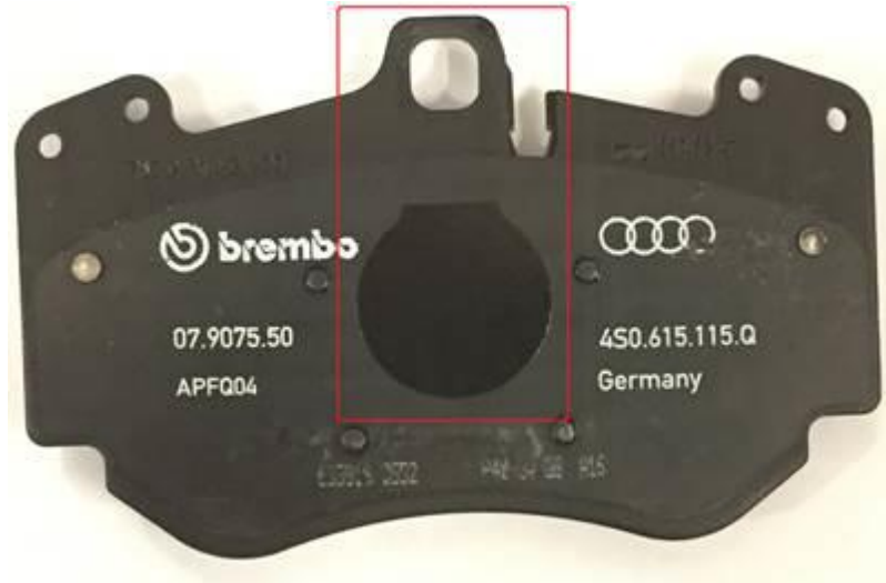
Figure 3. Do not touch the exposed adhesive surface.
