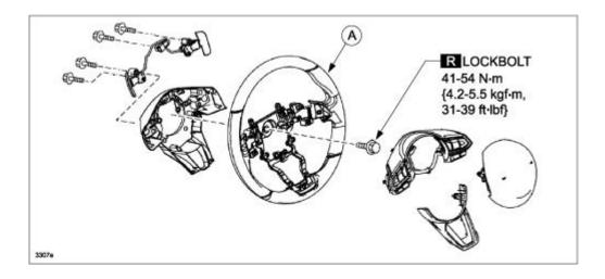
NOTE: For vehicles with a steering wheel warmer, replace the steering wheel hub kit (A).
