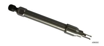
Figure 1. Injector Cup Tool
