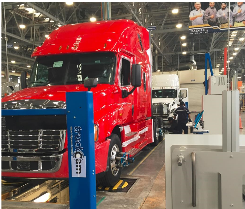
TruckCam™ Alignment System in Use at the Saltillo Mexico Plant
