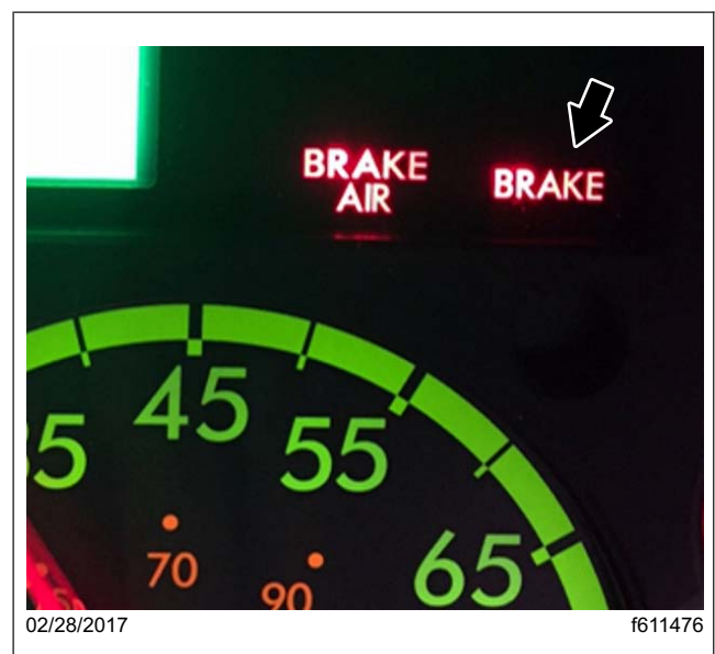
Fig. 2, A "Brake" Telltale is OK - No Replacement
