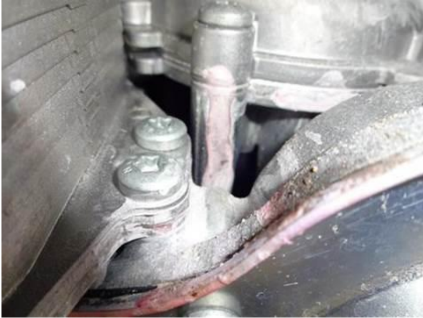
Figure 1. Coolant marks shown around coolant pump.
