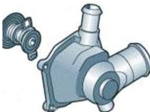
Figure 2. Coolant thermostat housing for map-controlled engine cooling.
