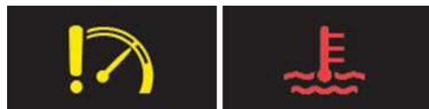
Figure 1. Engine speed governing light (left) and red coolant light (right).
