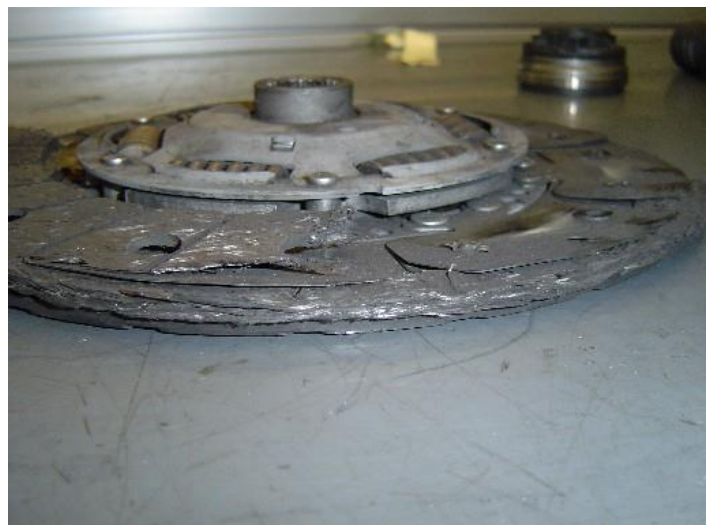
Figure 2. Burst lining from an overspeed condition.
