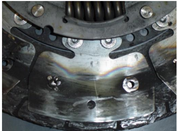
Figure 1. Lining partly removed due to overheating.
