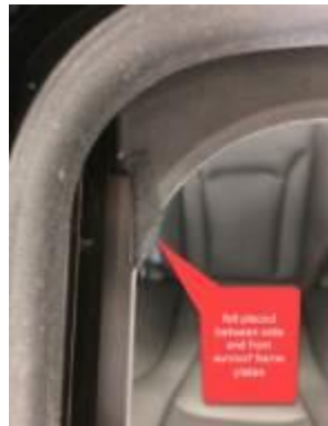
Figure 6. Fleece adhesive tape applied between the side and front sunroof frame plates.
