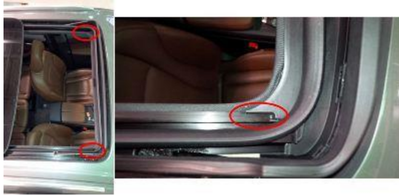
Figure 5. Areas of the sunroof frame to be isolated with fleece adhesive tape.
