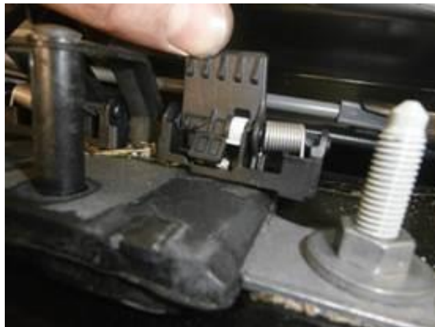
Figure 3. Debris in the Rear Lid Closed Sensor.
