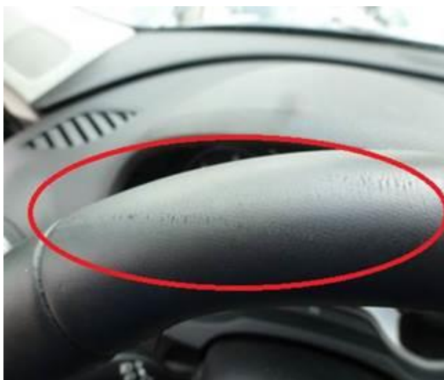
Figure 2. Example of damage from external impact.
