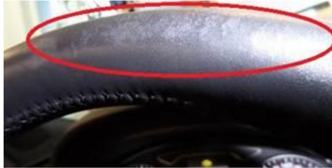
Figure 3. Example of damage from external impact.
