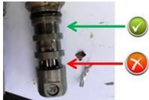
Figure 1. Two top filters are okay, bottom filter is missing.
