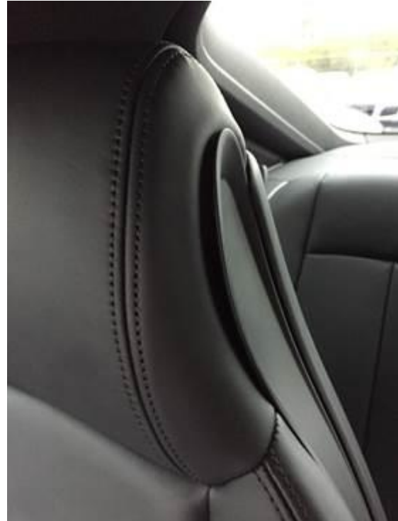
Figure 2. Inner front seat side trim loose.
