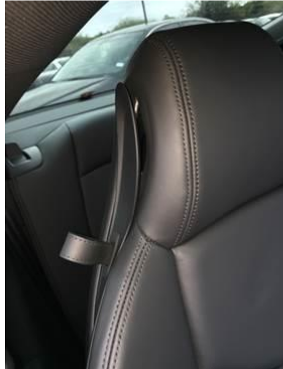
Figure 1. Outer front seat side trim loose.
