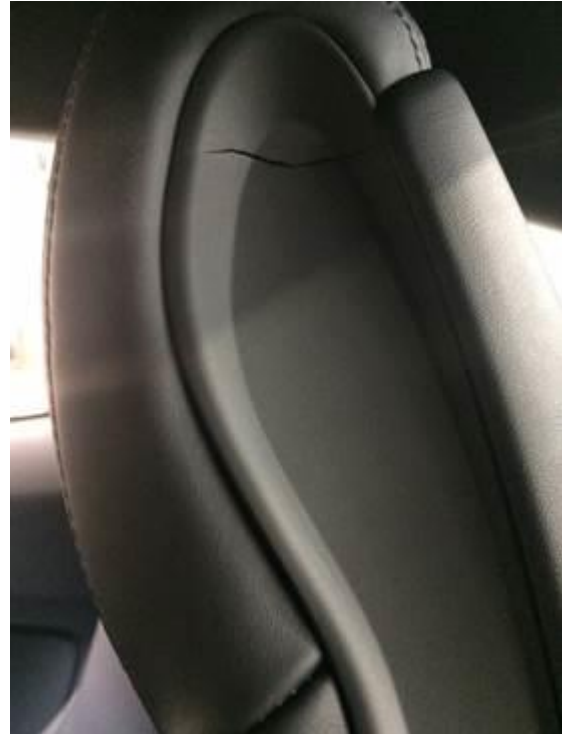
Figure 3. Front seat side trim cracked.
