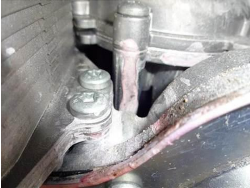
Figure 1. Coolant marks shown around coolant pump.
