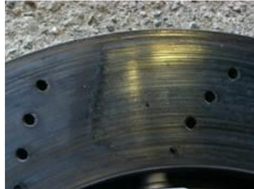
Figure 2. Deposits on the brake disc.
