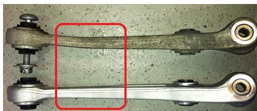
Figure 9. Damaged suspension link.
