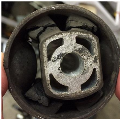
Figure 8. Damaged suspension bushing.
