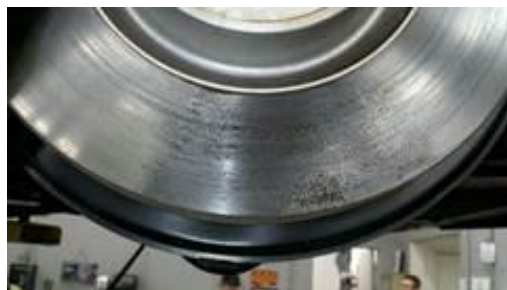
Figure 5. Pad marks on the brake disc.
