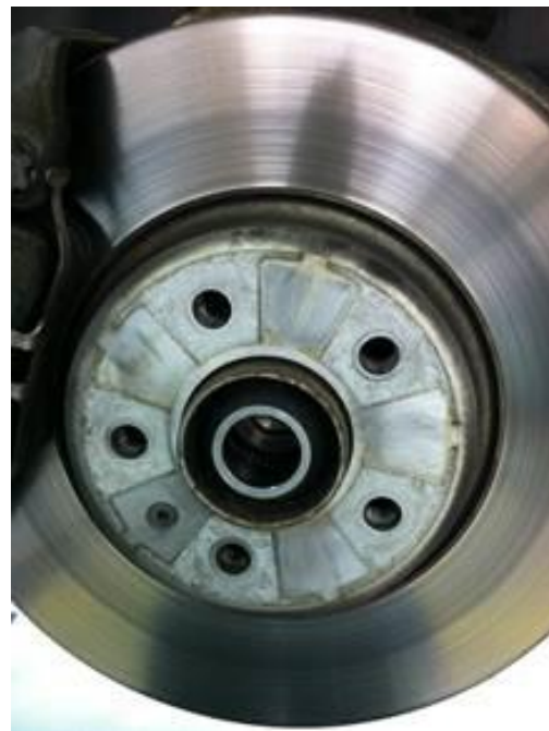
Figure 3. Brake disc with heat marks.
