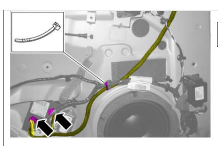
Caution! Ensure that the cable from the rear view mirror enters the connector from underneath.
