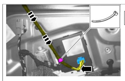
Caution! Ensure that the cable from the rear view mirror enters the connector from underneath.
