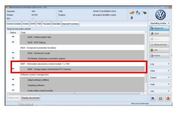
Under the Special Functions tab, run the "005F-Design status check/reset DTC memory" test plan.
