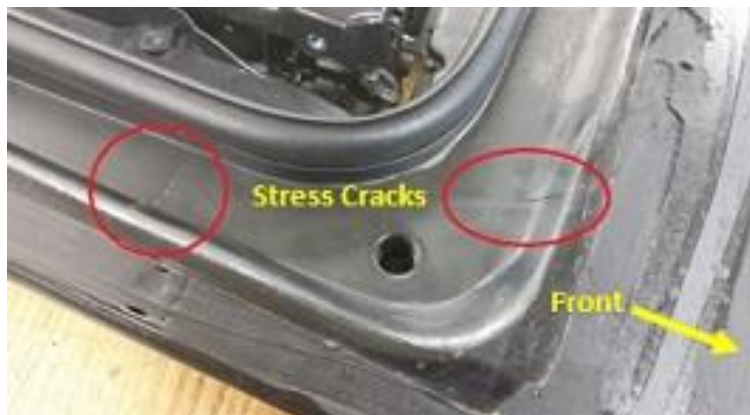
Figure 2 (Examples of stress cracks in water channel)
