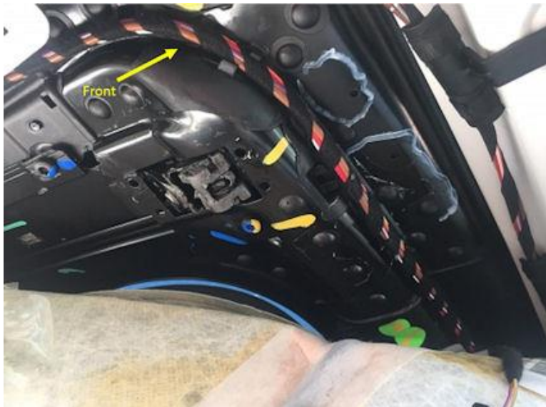
Figure 1 (Water leaking through corner of water channel)
