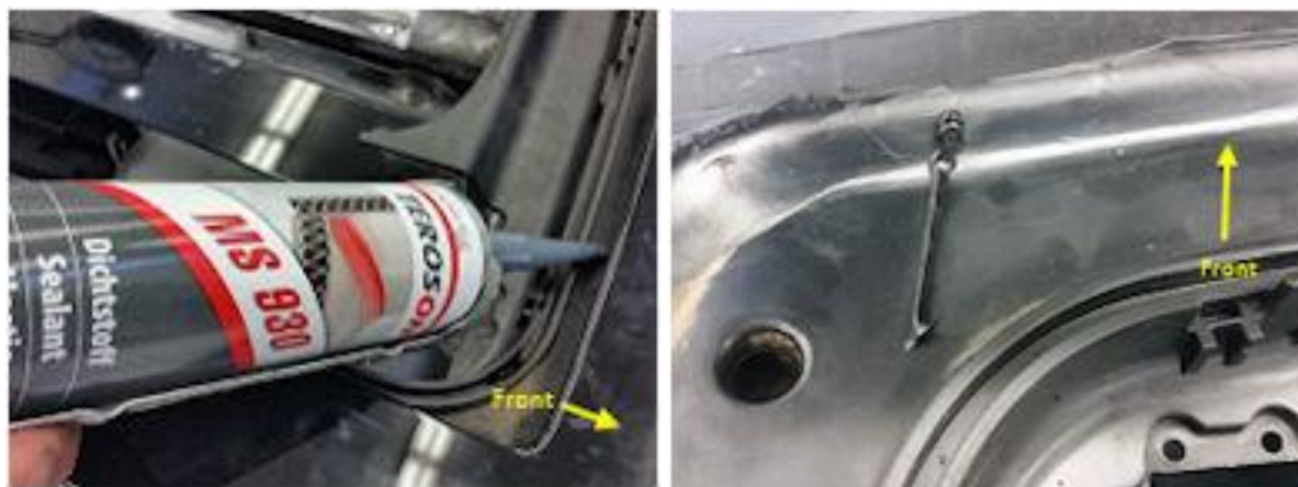
Figures 10 and 11 (Sealant application)
