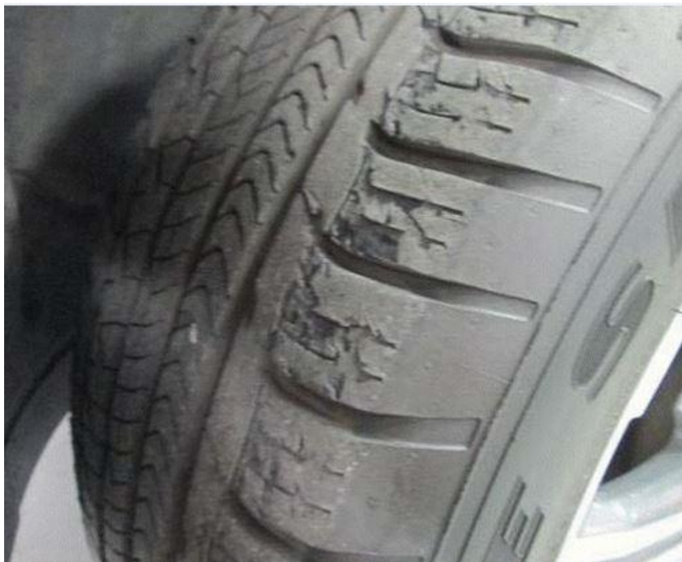
Figure 1. Irregularity on the outer side and on the inner side of the tire.
