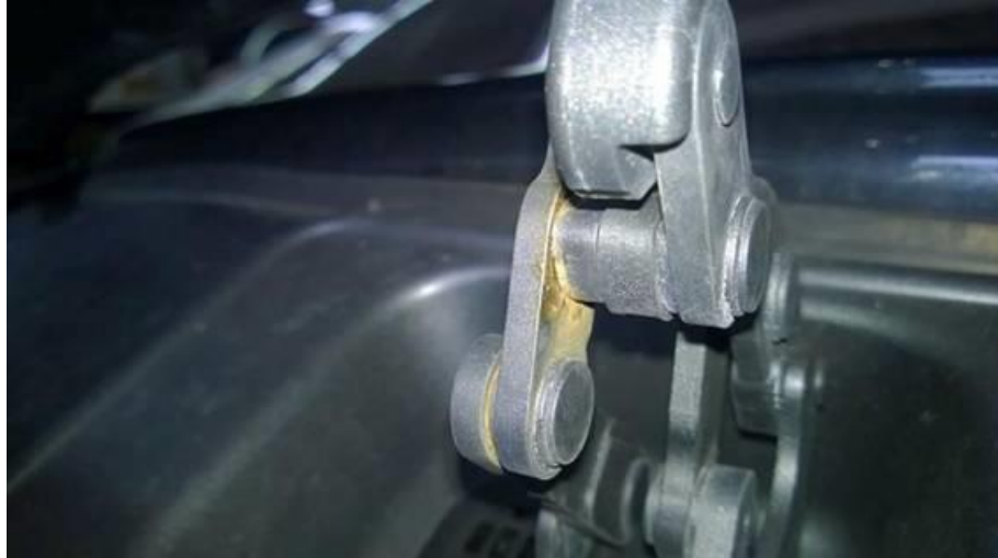
Figure 1. Corrosion on the spoiler drive unit hinge.
