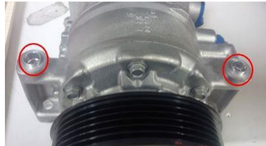
Figure 3. Mounting bolt centering sleeves on the air conditioning compressor housing.
