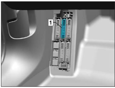
Pry out fuse carrier ST2 <1> using Trim Removal Wedge -3409- (or equivalent).
