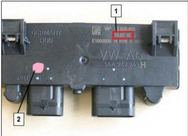
The control unit <1> must be replaced if it was manufactured within the following period:
