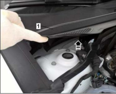
Press plenum chamber cover <1> slightly upwards in vicinity of suspension turret (right-side).
