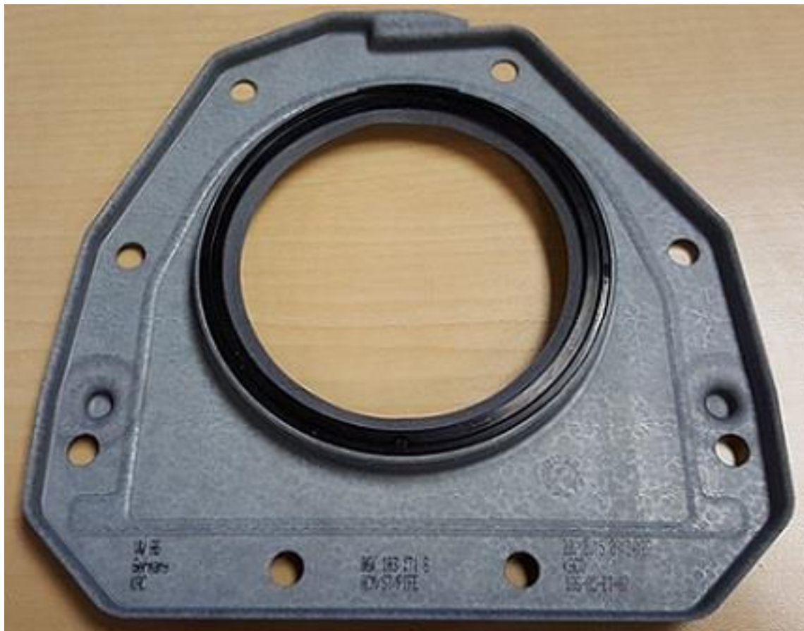
Figure 2. Front of sealing flange seal
