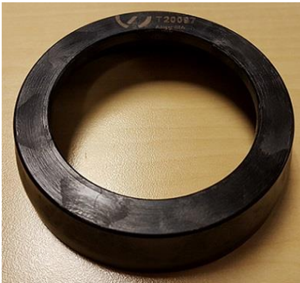
Figure 1. T20097 Sealing Flange Guide Sleeve
