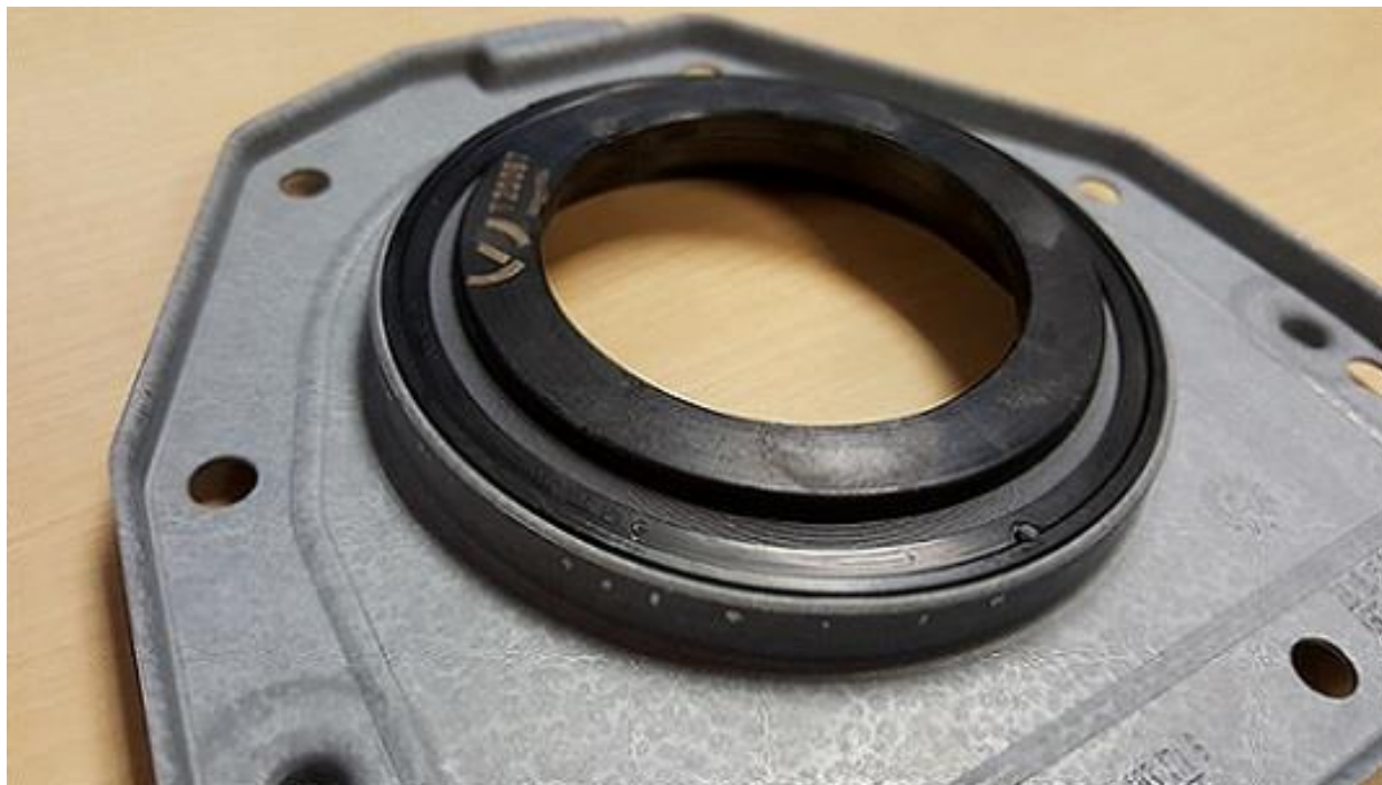
Figure 4. T20097 installed into the rear of the sealing flange seal
