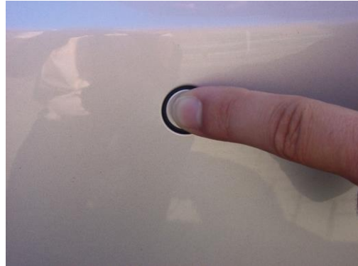
Figure 4. A pressure check on a parking aid sensor.
