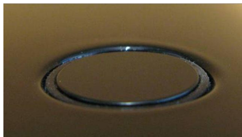
Figure 10. A correctly installed parking aid sensor.
