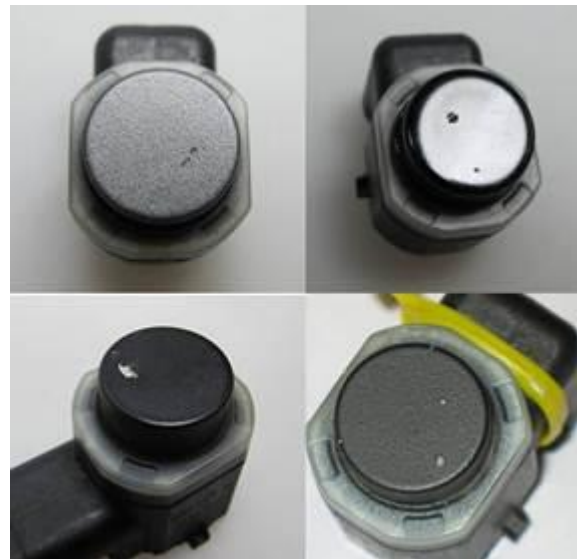
Figure 3. Stone chips causing sensor failure.
