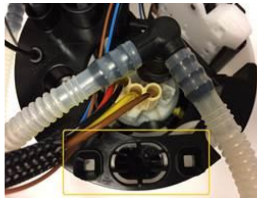
Figure 6. Install Control Valve “B”.
