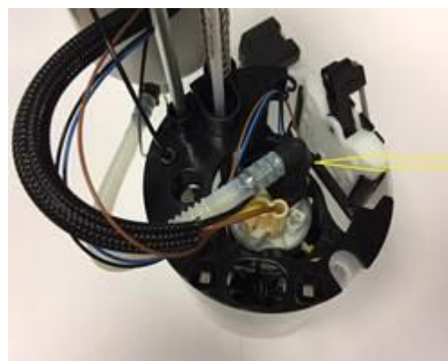
Figure 4. Disconnect the main supply line.
