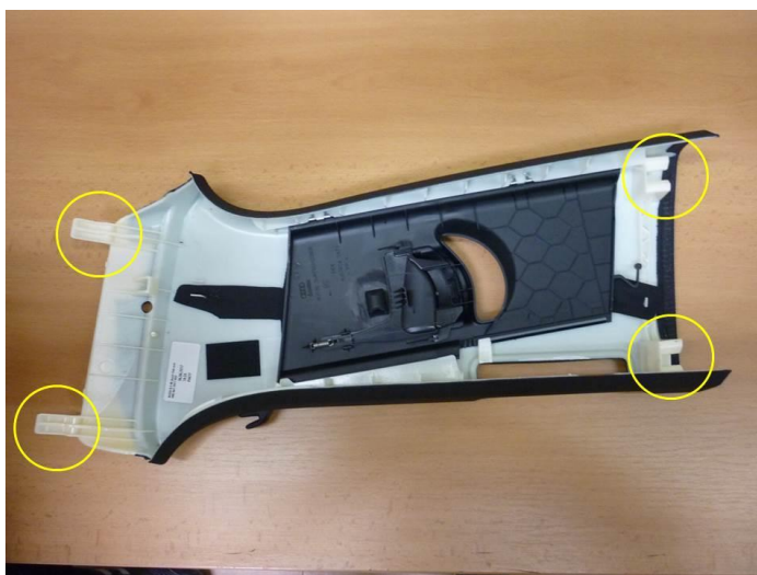
Figure 1. Mounting points of the B-pillar trim.
