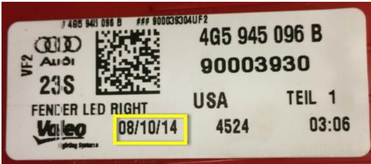
Figure 3. Location of production date, shown as DD/MM/YYYY. The production date of this taillight is October 8, 2014.
