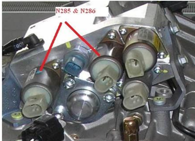
Figure 1. Gear selection valves N285 and N286.
