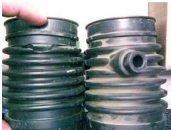
Figure 3. Crack in the intake hose.
