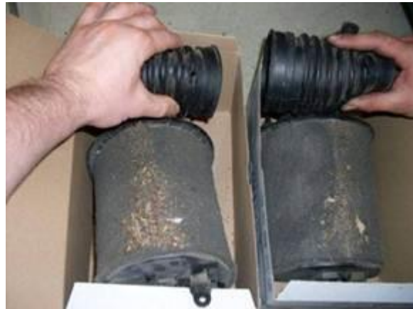
Figure 1. Example of excessive dirt on air filters.
