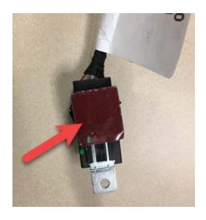
5. Mount the relay in the position shown below with the sticky tape
