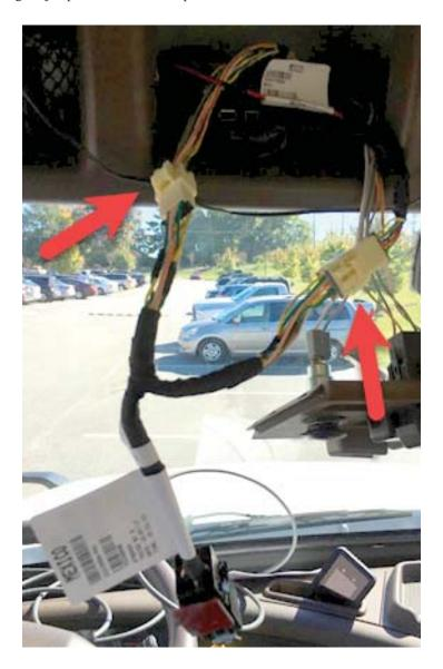
4. Remove the plastic from the sticky tape on the jumper harness relay
