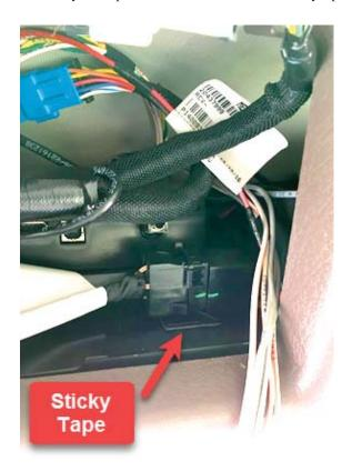
6. Secure the harness in the overhead using zip ties as necessary
