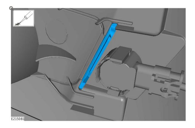
Apply a bead of sealant (Teroson® MS939, Loctite 5512™, or equivalent silane modified polymer sealant) to the areas shown.
