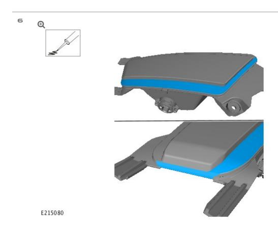
Apply a bead of sealant (Teroson® MS939, Loctite 5512™, or equivalent silane modified polymer sealant) to the areas shown.
