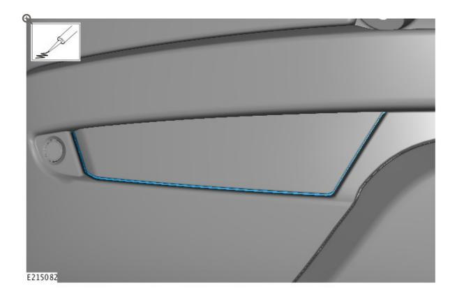
Apply a bead of sealant (Teroson® MS939, Loctite 5512™, or equivalent silane modified polymer sealant) to the areas shown.
