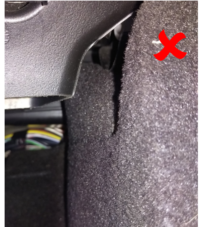
Carpet is turned back on its self, results in bulge and miss fit
