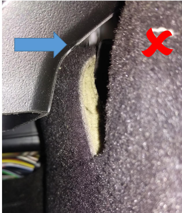
Top edge of carpet has entered the kinematic causing stall
