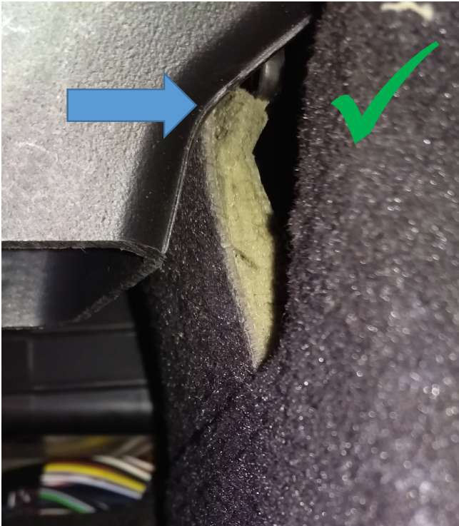
Carpet edge is vertical, end of carpet can be seen
