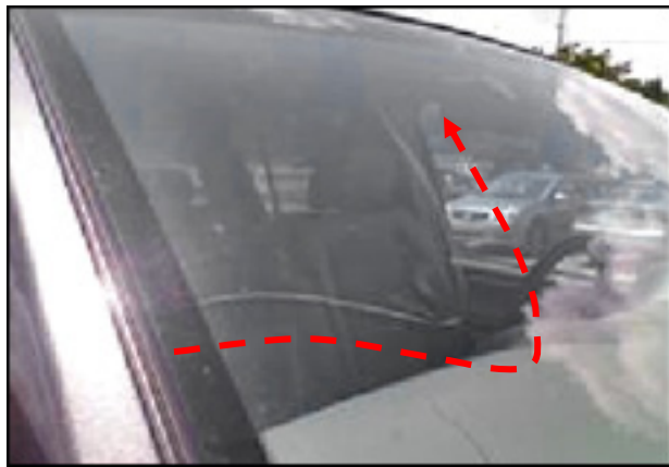
Single crack with no impact mark: Warranty
