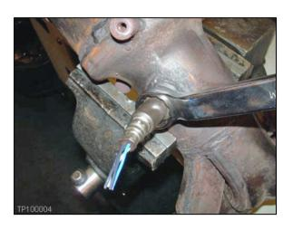
1. Clamp the exhaust manifold/catalyst/front tube in a vise.
