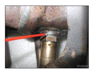
Continue the tightening/loosening motion while gradually unscrewing the sensor. Stop when the sensor will not unscrew any further.
