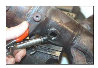
10. If metal debris remains trapped in the boss threads, use a spiral nylon brush to remove it.
