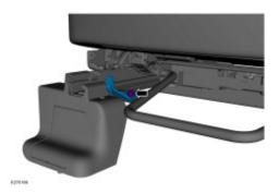
2. Move seat to the full rearward position and install the new seat track travel restrictor. Torque to 12 Nm (106 lb.in).
